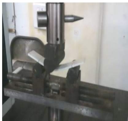
Figure.2. Tensile test (FRP2) Figure.3.Flexural test (FRP4) Figure.4.Shear test (FRP3)
