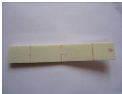
Figure.5.Tensile test specimen Figure.6.Flexural test specimen Figure.7.Shear test specimen
